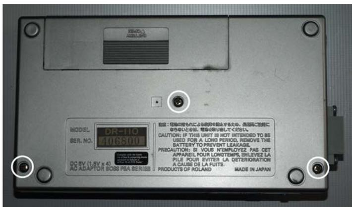
Remove the 3 screws on the base of the DR-110. The back should now come off. Set this aside for later.
