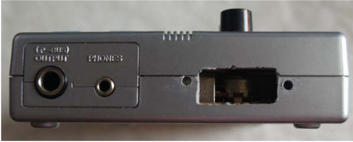
Remove a section of case and drill holes in order to fit the connector in the unit. The exact position may vary based on how the cable has been soldered so it is best to do this at this stage.
