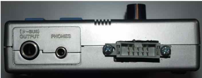
Use the nuts and bolt to secure the connector. Connect the DR-110 to the mod box.
