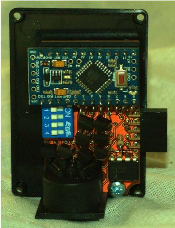
The final step is to affix the PCB to the enclosure. The controller chip will need to be removed for this.
