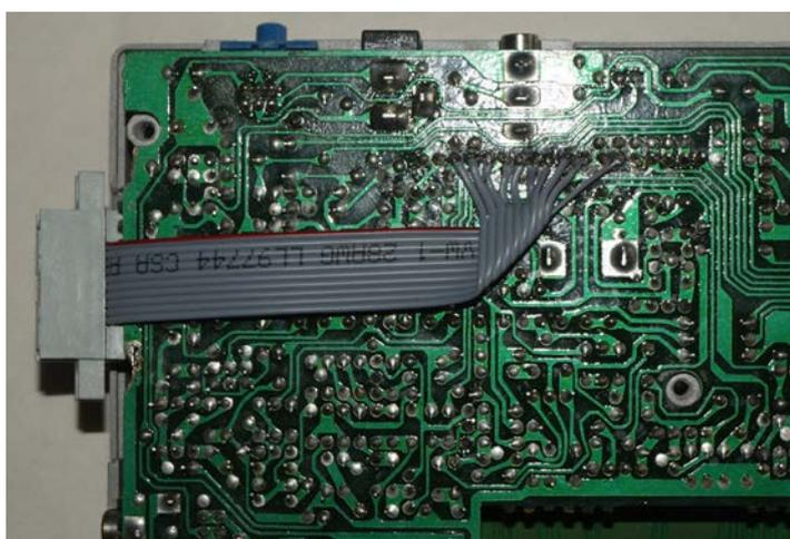
Once soldered, it should look similar to this. At this stage, it is a good idea to connect the mod to the unit to confirm it is working and triggering the sounds properly. If it is not, the soldering must be checked again and possibly redone.
